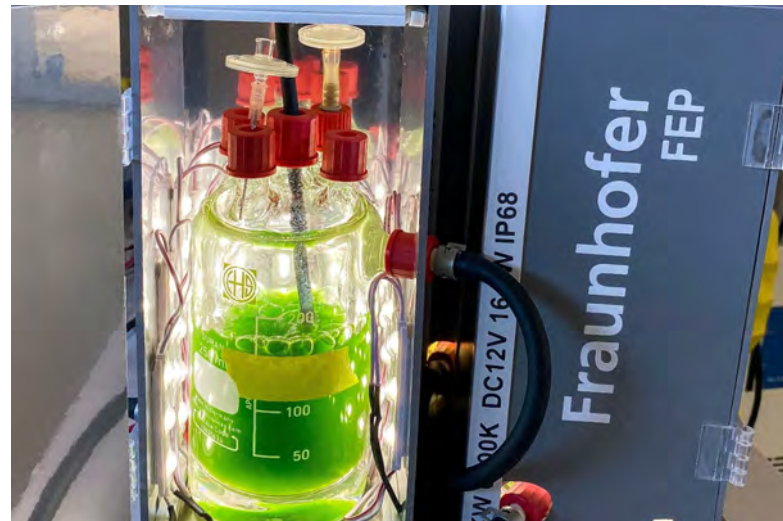
Modular cultivation system for phototrophic microorganisms for the production of secondary lime
