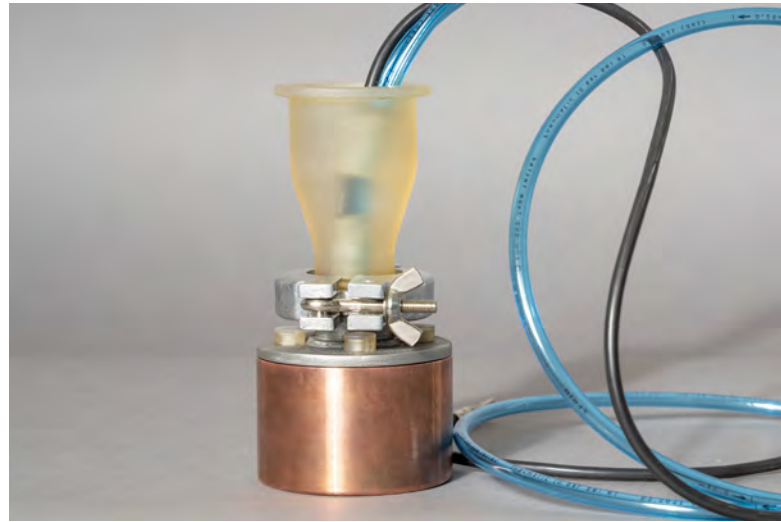
Magnetron sputtering source produced with additive manufacturing processes
