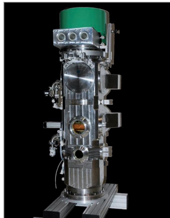
Fig. 1: Electron beam gun for deposition processes
