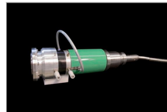
Fig. 2: Cold-cathode electron beam source
