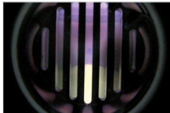
Fig. 1: View into the cathode compartment of an electron beam source, the cathode on top and anode-plasma at the bottom
