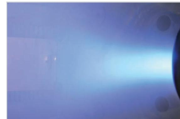
Fig. 3: View of a hollow cathode plasma source operating at 100 A discharge current and 100 V discharge voltage
