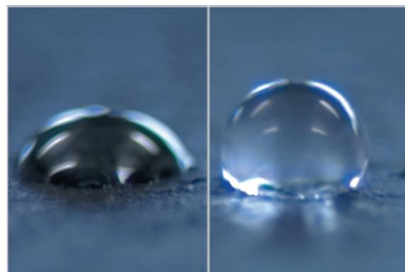
Fig. 3: Variable surface wettability after electron beam treatment
