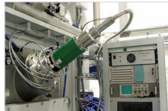
Fig. 2: Experimental 60 kW / 30 kV cold-cathode EB gun mounted to a pilot-scale coater
