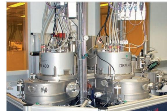
Fig. 4: Cluster-type sputter plant CS 400 S
