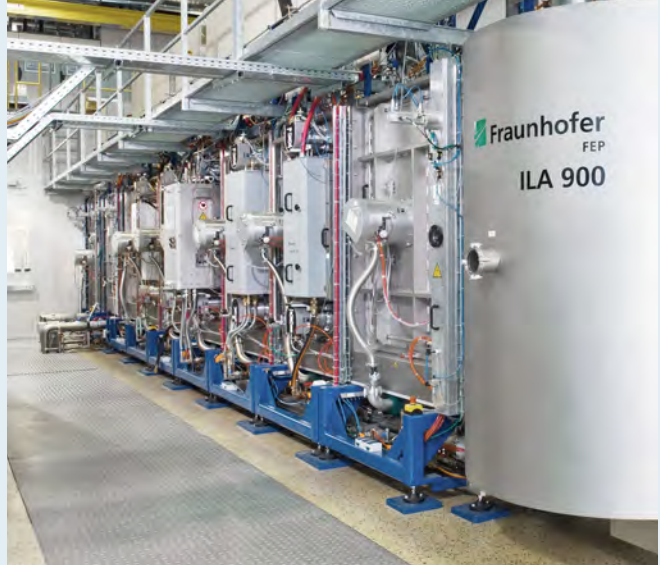
Vertical in-line sputtering for coating of large area surfaces
